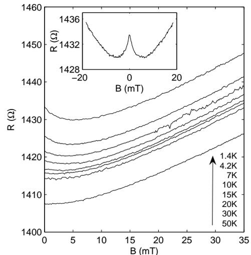
FIG. 1: Low-field magnetoresistance for a sample of 100  $\mu\text{m}$  by 1000  $\mu\text{m}$  at various temperatures. The inset: the magnetoresistance peak near  $B = 0$  can be seen when sweeping the field from -20 mT to 20 mT at 1.4K. The electron mobility is 11600  $\text{cm}^2/\text{V s}$ . The transport time  $\tau \sim 0.26$  ps is inferred from the resistivity.
