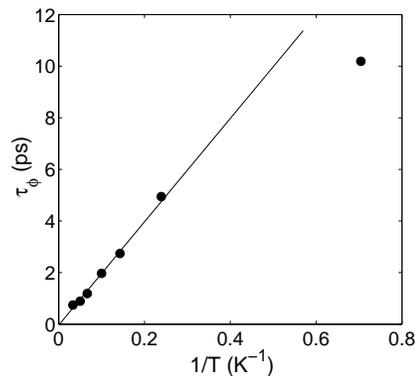
FIG. 3: Phase coherence time  $\tau_\phi$  as a function of inverse temperature  $1/T$ .  $\tau_\phi$  is obtained by a best fit to Eq. (1) for each temperature while  $\tau_{iv}$  and  $\tau_w$  are the same for all temperatures. Solid line is a guide to the eye.
